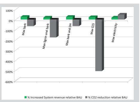
In a scenario with a high  $CO_2$  charge all of the technology pathways are profitable compared to business as usual (BAU), but the combination of maximum bark and district heating (DH) sales is the most profitable solution. The reduction of global  $CO_2$  emissions, however, varies and for increased electricity production the global emissions even increase.
